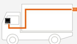
**Scope of delivery:** 5" digital colour LCD monitor, colour twin camera with shutter, 20 m connection cable from the monitor to the camera, monitor cable set, installation fittings for all components
