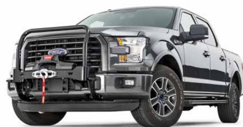
Ford F150, equipped with Gen II Trans4mer Mounting Kit and Grille Guard Tube (tall version)
