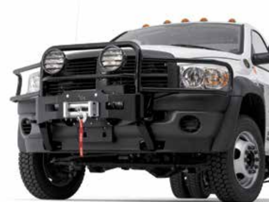
Ram HD equipped with WARN Gen II Trans4mer Mounting Kit, Grille Guard Tube (tall version), Headlamp Guards, and Light Bar
